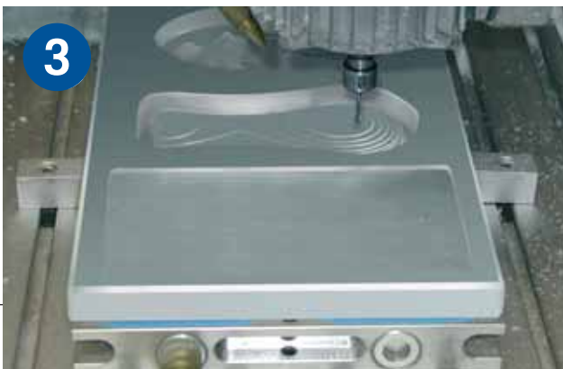
Right: After hardening, workpiece is turned over and machined on reverse side
