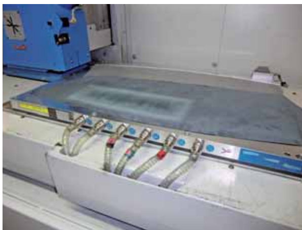
Application in automotive industry, leather clamped on visible side for grinding predetermined breaking points in areas of airbags on reverse side
