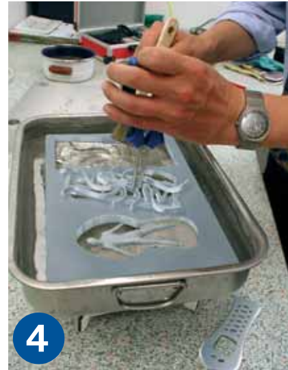
Top: Finally workpiece is placed in water at 80°C to melt and remove alloy, which can be reused
