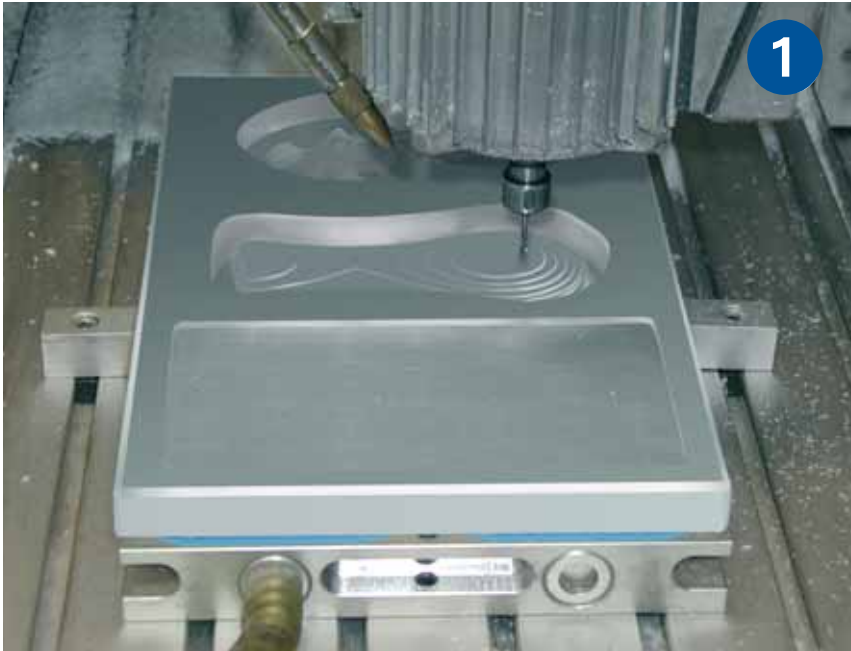
Left: First step is milling workpiece conventionally
