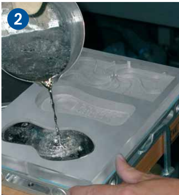
Right: Filling hollow with melted Witte Weiguss alloy
