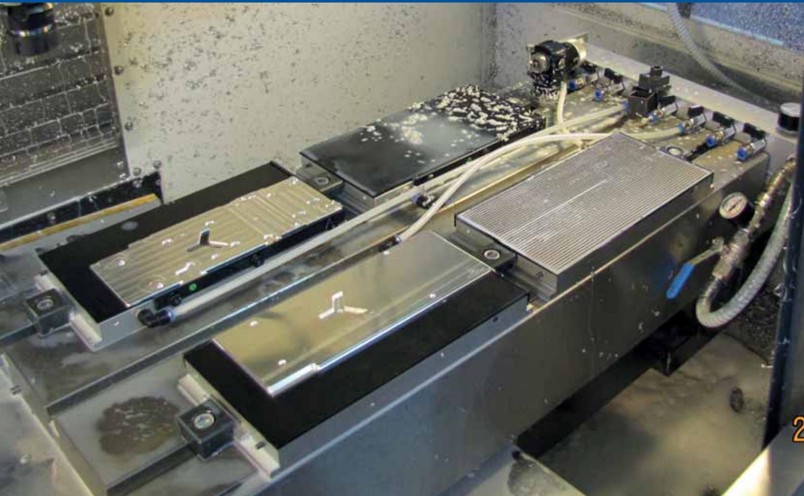
4 slot chucks on a machine used for manufacturing aluminium carriers. Machining of inner and outer contours is done in one process thanks to rubber adapter mats.
